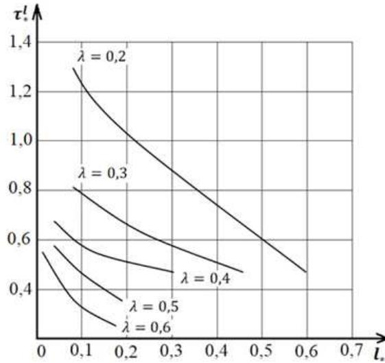
Fig. 6. Dependences of the critical load  $\tau_*^\ell = \tau_{xy}^\infty \sqrt{\omega} / K_{IIc}$  on the crack length in the inclusion
