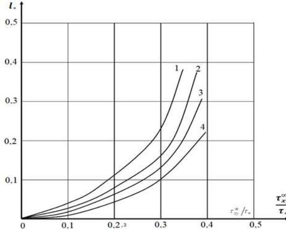
**Fig. 2. Dependences of the relative length of the pre-fracture zone  $l_* = (\ell - a) / \lambda$  on the dimensionless value of the external load  $\tau_{xy}^\infty / \tau_*$  for some values of the radius of the holes  $\lambda = 0, 2 \div 0, 5$  (curves 1 - 4)**
