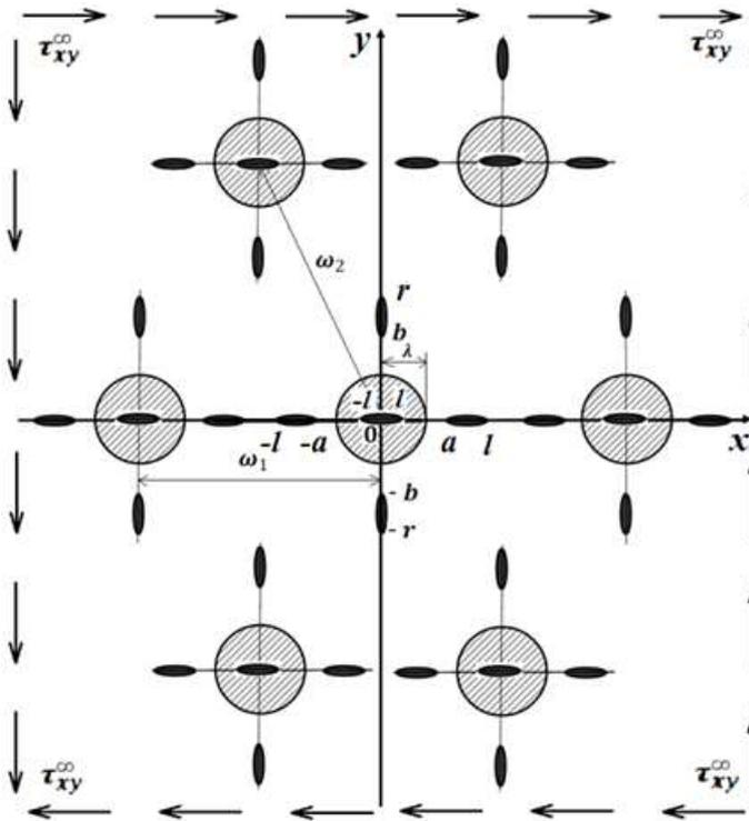
Fig. 1. Calculation scheme for the problem of crack initiation
