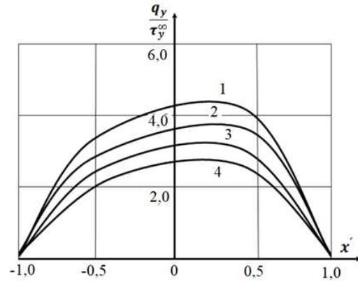
Fig. 3. Dependences of the distribution of shear stresses in the bonds  $q_x / \tau_{xy}^{\infty}$  along the pre-fracture zone for different values of the radius of the holes:  $\lambda = 0, 2 \div 0, 5$  (curves 1 - 4)
