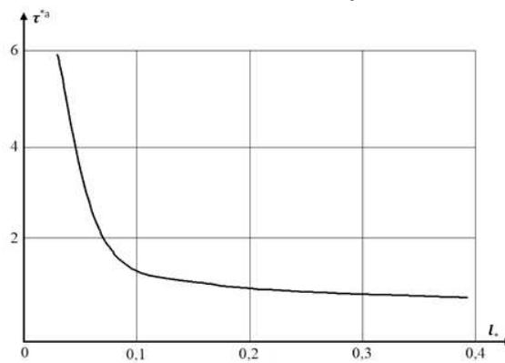
Fig. 5. Dependence of the critical load  $\tau^{*a} = \tau_{xy}^{\infty} / \tau_*$  with a change in the length of the pre-fracture zone  $l_* = l - a$  at  $\lambda = 0, 3$ ,  $a_* = 0, 05$
